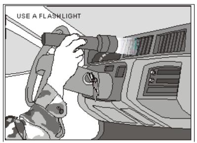
Use a flashlight to check the air conditioning ducts and other vehicle cavities.
