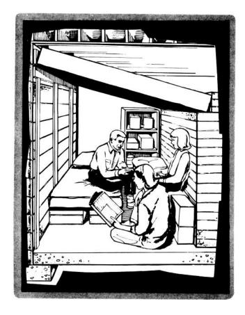
A storage unit is hinged to the wall in a basement corner. It is tilted-up to rest on stacked brick or concrete block and filled for overhead protection.
