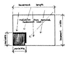
If it is found to be impractical to shield one quarter of the basement ceiling area, the extent of ceiling modification may be reduced to any desired size by constructing vertical masonry walls on the two open sides of the shielded area, thus providing a room suitable for use as a hobby or laundry room. These masonry walls will also provide protection from excessive amounts of radiation coming through exposed portions of the basement wall.
