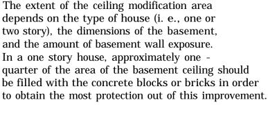
This arrangement will effectively shield all of the radiation coming from the roof - the largest contributing source.
