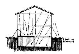
In homes with 2 or more stories above ground, the extent of the basement ceiling modification can usually be reduced to 12' x 12'. Note, however, that vertical side walls may be required if the basement wall exposure exceeds two feet.
