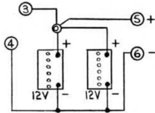
Batteries may be wired in parallel to increase capacity.
