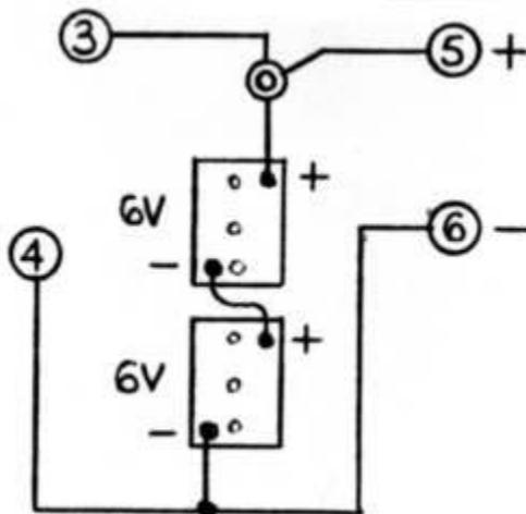
Batteries are wired in series to increase voltage.
