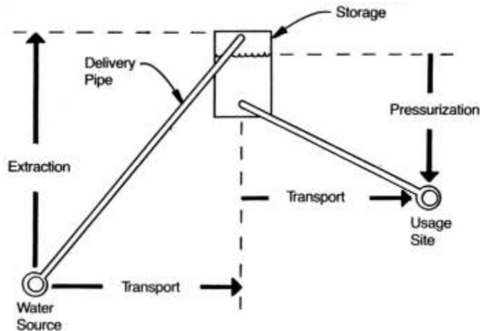
Water systems involve the processes of extraction, transport, storage, and pressurization.
