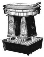
Fig. 94. Device for distilling sulphur in greenhouses
