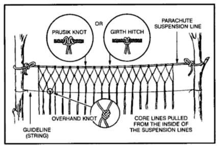
Figure 8-19. Making a gill net.
