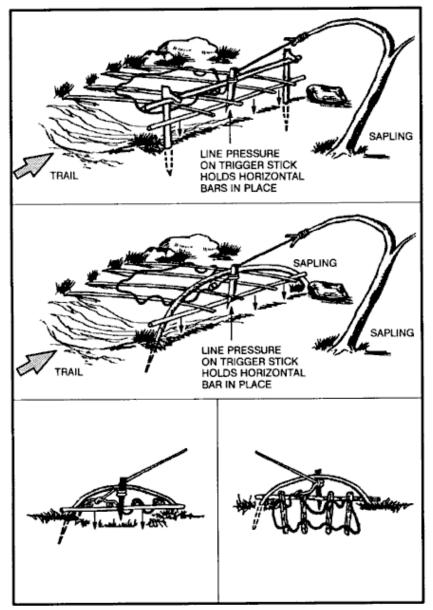
Figure 8-11. Treadle spring snare.
