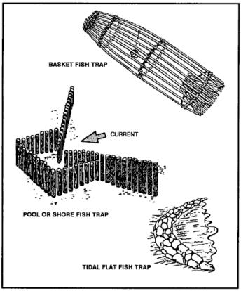
Figure 8-21. Various types of fish traps.
