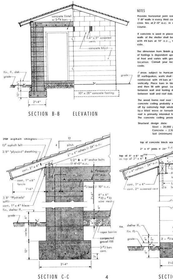
Provide horizontal joint reinforcement for 1'-8" walls in every third course and metal cross ties at 2'-0" o.c. in every alternate
