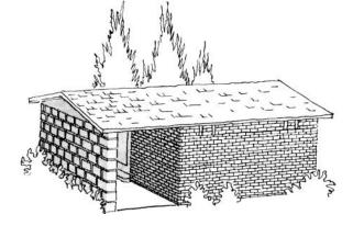
SECOND ALTERNATE shows the cement block faced with bricks. Use one course 4-inch brick and two courses of 8-inch cement block to obtain the required weight per unit area.
