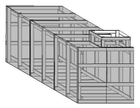
Once the frame is complete, your panels can be fastened to the frame. Do one end first, then the sides, working from one end to the other.
