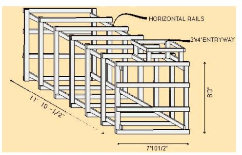
The box, as shown in Figure 1, is made up of five ribs, and two ends.
