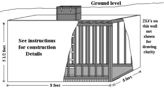
**Underground Storage Room, Cutaway View**
